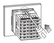
\*Mount the product on the panel, fasten bracket by pushing with tools as shown above.
