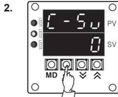
C-5u is displayed in the PV display part, 0 is displayed in the SV display part. Press the **←** key (S2).
