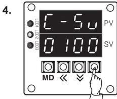
Press the **→** key (S4) and set 1 at 10<sup>2</sup> digit and press the **MD** key.
