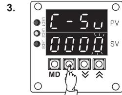
10<sup>0</sup> digit flashes in the SV display part. Move the digit by pressing **←** key (S2) twice.
