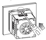
Mount the product on the panel, fasten bracket by pushing with tools as shown above.
