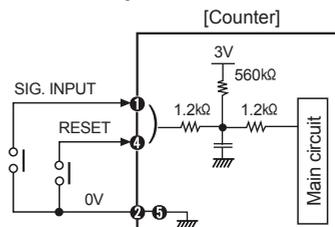
※When power is applied to terminal No ① and ②, input terminal circuit can be broken and a malfunction can occur.
