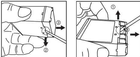
※Hold up Lock part toward ①, ② of the product with the tool and pull toward ③ to detach the case.
