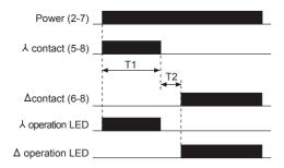
$\mbox{\em XT2:}\ \mbox{\em $\lambda$}$  switching time ( $\mbox{\em $\lambda$}$  contact are OFF simultaneously at power ON)
