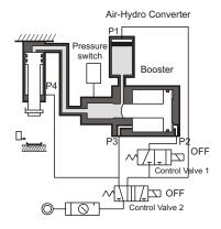
When the air is send into port P4 and P3. the hydraulic cylinder is swiftly reversed. and at the same time the ram goes back.
