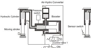
When the air is charged from the port P1, the oil in the tank will forward the hydraulic cylinder quickly. The pressure is the same as the air pressure, but the inflow of oil is large in volume.
