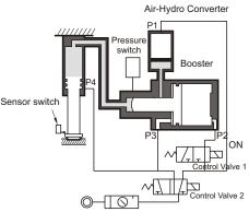
When the air is charged from the port P2, a ram will advance. the highly pressured fluid will come in to the hydraulic cylinder which will be forwarded by large thrust.
