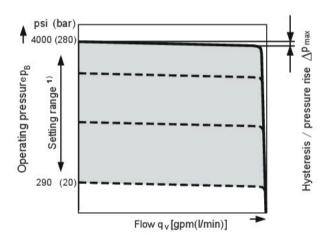
1) In order to prevent damage to the pump and the system, this setting range is the permissible setting range and must not be exceeded.
