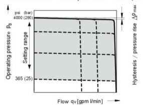
1) In order to prevent damage to the pump and the system, this setting range is the permissible setting range and must not be exceeded. The range of possible settings at the valve are greater.
