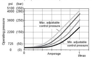
Hysteresis static current-press. characteristic < 45 psi (3 bar) Influence of pressure setting on stand-by ±30 psi (±2 bar)
