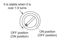
Put the object in right sensing position, turn the potention VR to the left and stop at the proximity sensor is OFF(ON).
