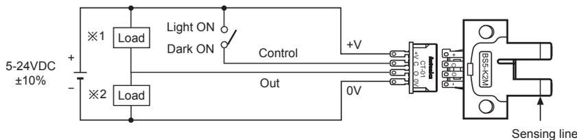
※1: The load connection of NPN open collector output
