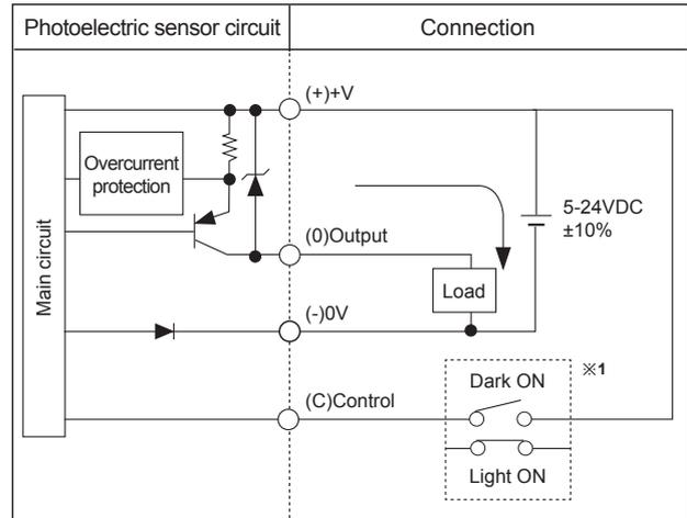
※1: Operation mode selection : Connect Control(C) terminal into terminal +V(+) to operate Light ON mode.
