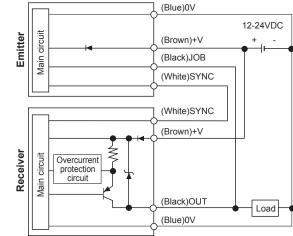
% If the receiver OUT(Black) line and the emitter JOB(Black) line are not connected each other, the JOB indicator of the emitter is not operated and maintain the light status.
