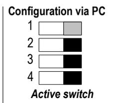
**Caution:** the configuration of the parameters can be done either with the DIP switch or via software (you can not combine both solutions).
