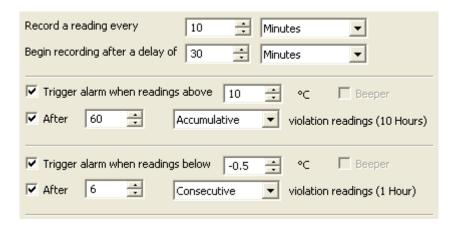
**Note:** Accumulative or consecutive alarms automatically retrigger after the configured delay if the temperature remains in violation.
