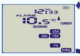
The temperature excursion has triggered an alarm.
