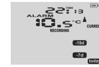
10 hours later the over temperature duration triggers an alarm. The **ALARM** symbol and the **today** marker are shown.
