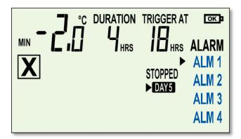
Example of an alarm display for above alarm limits.
