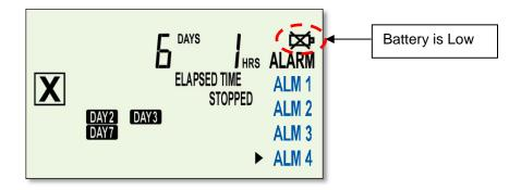
An Indicator should not be used if it shows the low battery symbol at the beginning of a trip. Indicators with a low battery not yet recording cannot be started.
