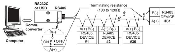
※ It is recommended to use Autonics communication converter; SCM-US48I (USB to RS485 converter, sold separately), SCM-38I (RS232C to RS485 converter, sold separately). Please use twisted pair wire for RS485 communication.
