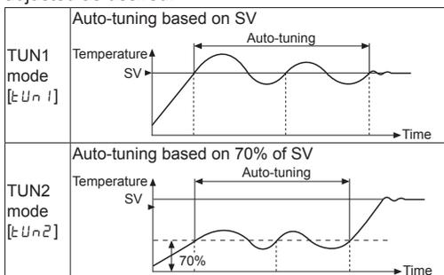
To manually stop auto-tuning, hold the [AT] key for 5 seconds. When auto-tuning is stopped, the controller maintains the PID value before auto-tuning. TZ Series supports 2 auto-tuning modes.
