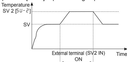
E.g.) The internal temperature of an electric oven may drop rapidly if the door is opened while the oven is maintaining a specific temperature. Set SV2 temperature [SV-2] to a higher value than SV, and input a signal to the external terminal (SV2 IN), to quickly raise the temperature.
