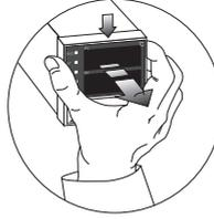
Press the front case then pull the case to detach the case from the body. Configure the internal switches as input type.
