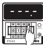
※ Set the position of decimal point using  $\uparrow$ ,  $\downarrow$  button of digital switch.
