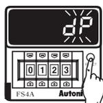
※ When "dP" is flashing, one touch the Reset button.
