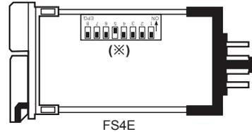
※In case of indicator (FS5E1), 5 Pin DIP switch is included, because there is no output operation mode.
