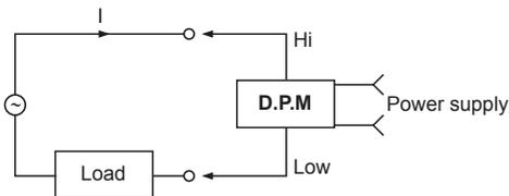
(Fig. 3) Measuring lower than AC5A of current
