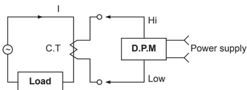
(Fig. 4) Measuring higher than AC5A of current
