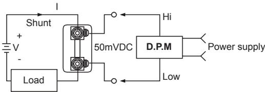
(Fig. 2) Measuring higher than DC2A of current
