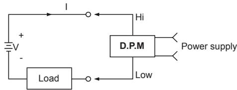
(Fig. 1) Measuring lower than DC2A of current
