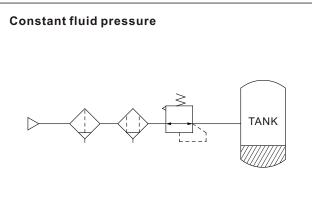
% Since there is a large effective area for supply and exhaust, pressure setting can be done quickly.
