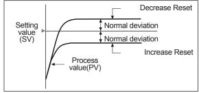
Manual reset function is applicable only to P / PD control mode.
