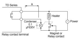
Keep power relay as far away as possible from temperature controller. If wires length of **A** is short, electromotive force occurred from a coil of magnet switch & power relay may flow in power line of the unit, it may cause malfunction. If wires length of **A** is short, please connect a mylar condenser 104(630V) across coil of the power relay "" to protect electromotive force.
