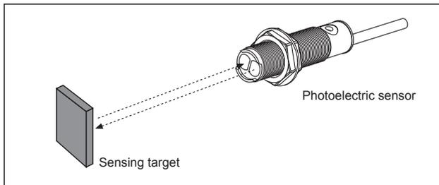
2. Set the target at a position to be detected by the beam, then turn the adjustment VR until position ㉑ where the operation indicator turns ON from min. position of the adjustment VR.
