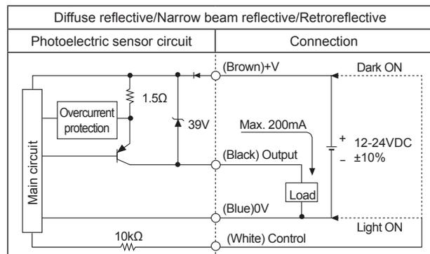
※ Before using this unit, select Light ON/Dark ON with control cable. (Light ON : Connect control cable with 0V / Dark ON : Connect control cable with +V)
