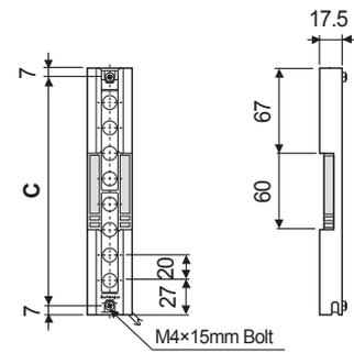
※ It is able to mount parallel or L-shaped bracket together.
