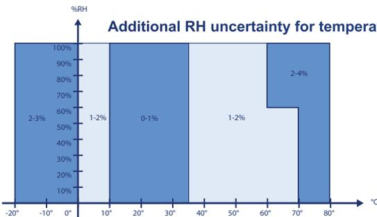
This graph shows the possible additional uncertainty in %RH compared to the accuracy specifications for temperatures different than 25°C for the standard factory calibration. The shown uncertainties may be positive or negative.
