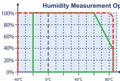
This chart shows the normal recommended operating range of the humidity sensor. Conditions outside the recommended range may temporarily offset the RH signal up to ±3 %RH.
